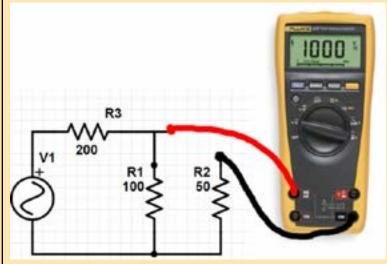
Here we wish to measure the current in the leg of the circuit containing R2. To do this we open the circuit and insert the meter in series.
