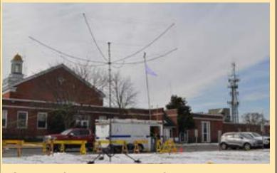
Our simplified setup: two end-fed antennas and the BuddiHEX. We can pull up anywhere and be on the HF bands pretty fast.
