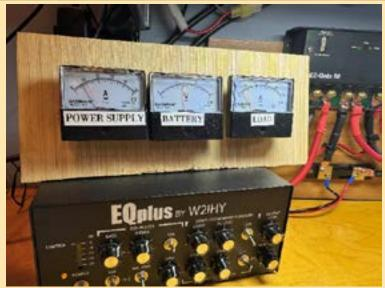
In the picture above, you can see the three meters I installed. Below, you can see the shunts for amperage meters. You can also see the 4-gauge wiring that I ran. So far, so good: All works really well now.
