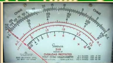
is across all components connected in parallel). Because the meter has a very high resistance only a small amount of current is drawn away from the circuit to make the measurement. If we connected a small resistance we would change the total circuit resistance, downward, resulting in the circuit experiencing 'loading' and more current flow. We want to affect the circuit as little as possible.
