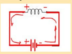
There is a tiny voltage drop across the inductor due to the resistance (miniscule but measurable) of the wire.
