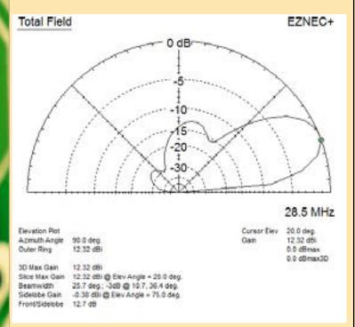
Analyzing the combined beamwidth figures we see that this antenna puts out its main power with a horizontal width of 65.8 degrees and a vertical beamwidth of 25.7 degrees centered on an elevation of 20 degrees above the horizon.
