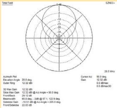
This is a directional antenna, so most of the gain is in a single direction. In this azimuth plot the elements are from left to right with the direction of gain being to the top of the
