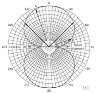
This is the pattern looking down from above the wire which is suspended from left to right. The outer circle of the diagram is drawn where the gain is at maximum and is labeled 0dB. This is the maximum gain of the antenna. 0dB represents a multiplication factor of 1, or 100%. All other circles inside the outer 0dB circle represent less gain and are labeled as negative decibel units (i.e., loss) to reflect this.
