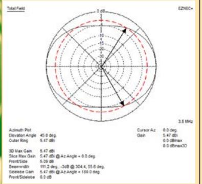
The azimuth pattern shows us that the maximum gain is at 0.0 degrees (and also 180 degrees opposite) with an azimuth beamwidth of 111.2 degrees at 304.4 and 55.6 degrees. I've added a dashed circle at the -3dB ring and a set of arrows pointing to where the pattern crosses the -3dB points. The beamwidth is between those arrows.
