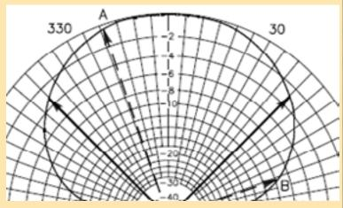
Each of the azimuth lines here represents 5 degrees and we have 45 degrees to each side for a beamwidth of 90 degrees.
