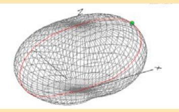
The modeling software automatically selects the slice with the maximum gain for the plots. The dipole wire in these plots is along the Y-axis which is from top to bottom in the 2D plots or the Y-axis in the 3D plots.
