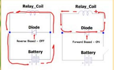
On the left we can see the diode is reverse biased and so does not conduct. All the current flows through the coil, back to the battery. On the right the circuit from the battery is opened allowing the coil to discharge. When the coil discharges it becomes a current source like the battery with a polarity reversal that now forward biases the diode allowing current to flow freely back to the inductor.
