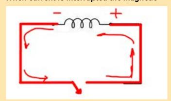
field collapses and its polarity reverses to become a current source.
